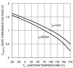
Figure 8. Gate Threshold Variation vs. Temperature
