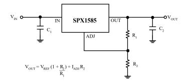
Fig. 5 Typical Adjustable Regulator
