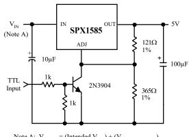
Note A:  $V_{IN(MIN)} = (Intended V_{OUT}) + (V_{DROPOUT (MAX)})$
