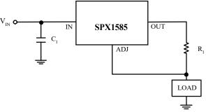
Fig. 4 5A Current output Regulator
