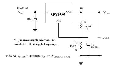
Fig. 6 Improving Ripple Rejection
