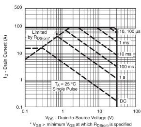
\*  $V_{GS}$  > minimum  $V_{GS}$  at which  $R_{DS(on)}$  is specified **Safe Operating Area**
