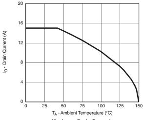
Maximum Drain Current vs. Ambient Temperature
