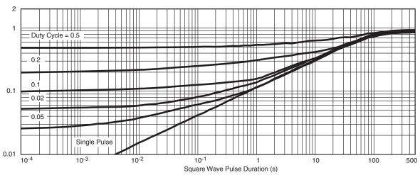
Normalized Thermal Transient Impedance, Junction-to-Ambient
