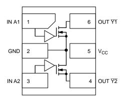
Figure 1. Pinout (Top View)
