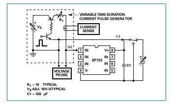
Figure 5: SP723 Typical Single Peak Current Pulse Capability
