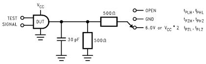
FIGURE 1. AC Test Circuit
