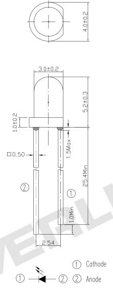
Note: Tolerances unless dimensions ±0.25mm
