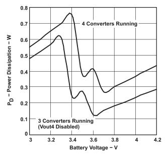
Figure 18. Power Dissipation vs Battery Voltage
