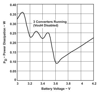
Figure 19. Power Dissipation vs Battery Voltage
