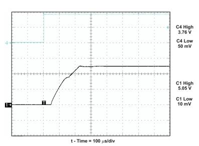
TEST CONDITIONS  $V_I = 3.7 \text{ V}$ EN1 = 0 V to 3.7 V
