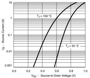
Source-Drain Diode Forward Voltage
