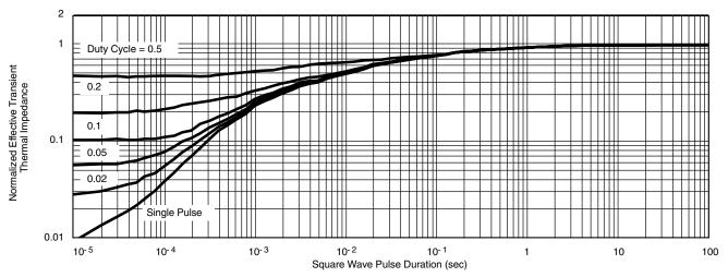
Normalized Thermal Transient Impedance, Junction-to-Case
