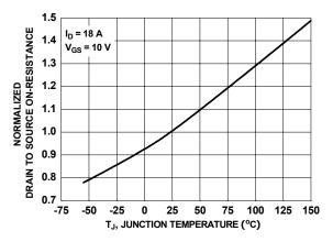
Figure 3. Normalized On-Resistance vs Junction Temperature
