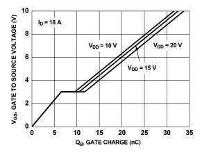
Figure 7. Gate Charge Characteristics
