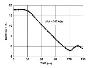
Figure 14. FDMS7672AS SyncFET body diode reverse recovery characteristic
