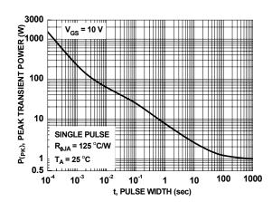
Figure 12. Single Pulse Maximum Power Dissipation
