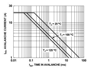
Figure 9. Unclamped Inductive Switching Capability
