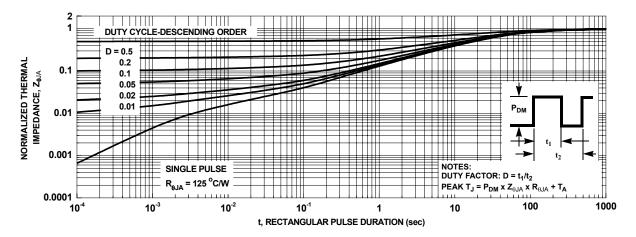
Figure 13. Junction-to-Ambient Transient Thermal Response Curve
