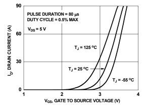
Figure 5. Transfer Characteristics
