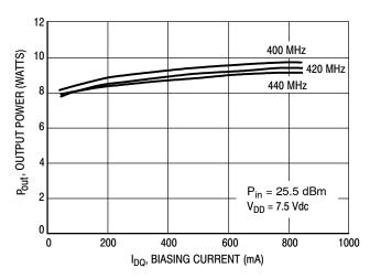
Figure 15. Output Power versus Biasing Current
