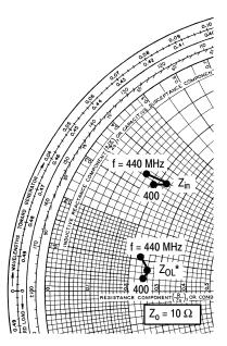
$V_{DD}$  = 7.5 V,  $I_{DQ}$  = 150 mA,  $P_{out}$  = 8 W
