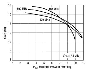
Figure 4. Gain versus Output Power
