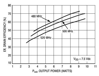
Figure 5. Drain Efficiency versus Output Power
