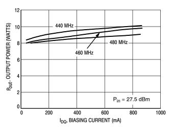
Figure 24. Output Power versus Biasing Current
