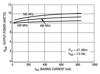
Figure 6. Output Power versus Biasing Current
