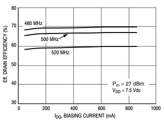
Figure 7. Drain Efficiency versus Biasing Current
