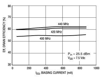
Figure 16. Drain Efficiency versus Biasing Current
