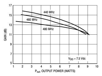
Figure 22. Gain versus Output Power
