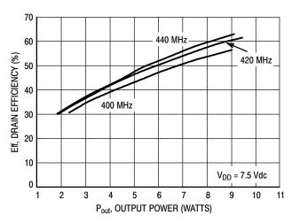
Figure 14. Drain Efficiency versus Output Power
