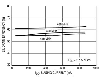
Figure 25. Drain Efficiency versus Biasing Current
