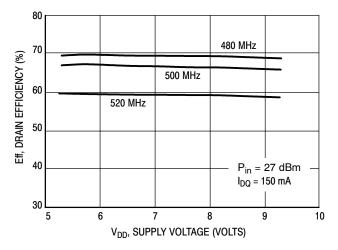
Figure 9. Drain Efficiency versus Supply Voltage
