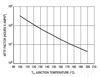
This above graph displays calculated MTTF in hours x ampere<sup>2</sup> drain current. Life tests at elevated temperatures have correlated to better than  $\pm 10\%$  of the theoretical prediction for metal failure. Divide MTTF factor by  $I_D{}^2$  for MTTF in a particular application.
