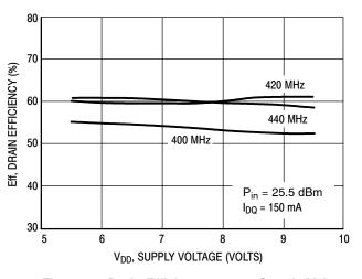
Figure 18. Drain Efficiency versus Supply Voltage
