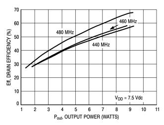
Figure 23. Drain Efficiency versus Output Power
