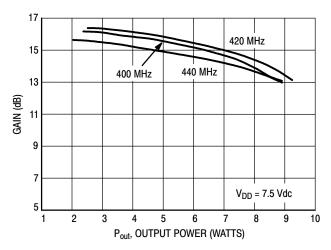
Figure 13. Gain versus Output Power
