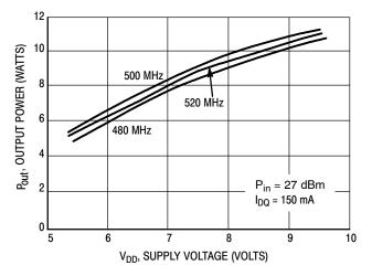
Figure 8. Output Power versus Supply Voltage
