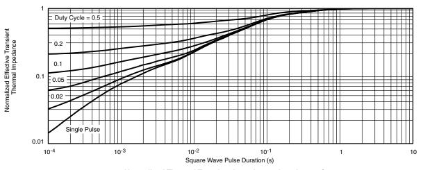
Normalized Thermal Transient Impedance, Junction-to-Case
