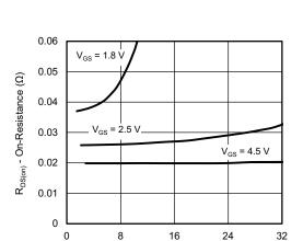
On-Resistance vs. Drain Current and Gate Voltage
