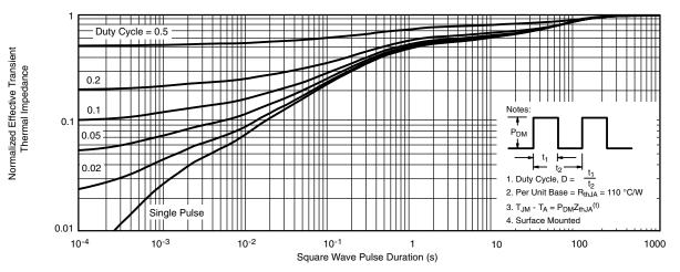
Normalized Thermal Transient Impedance, Junction-to-Ambient
