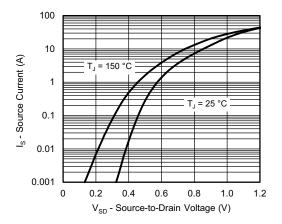
Source-Drain Diode Forward Voltage
