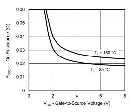
On-Resistance vs. Gate-to-Source Voltage
