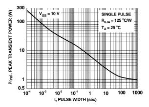
Figure 12. Single Pulse Maximum Power Dissipation
