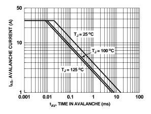
Figure 9. Unclamped Inductive Switching Capability
