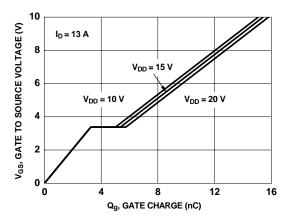
Figure 7. Gate Charge Characteristics
