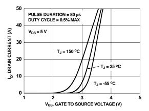
Figure 5. Transfer Characteristics
