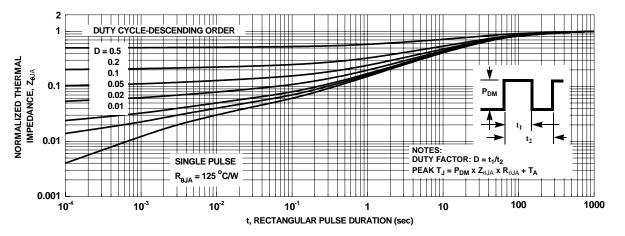
Figure 13. Junction-to-Ambient Transient Thermal Response Curve
