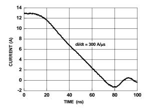
Figure 14. Body Diode Reverse Recovery Characteristics
