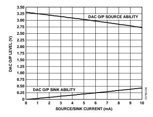
Figure 23. DAC Source and Sink Current Capability
