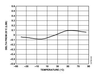
Figure 10. Change in ADC Offset vs. Temperature
