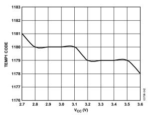
Figure 19. Temp1 vs. Vcc
