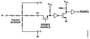
Figure 43. PENIRQ Output Equivalent Circuit
