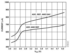
Figure 7. Supply Current vs.  $V_{CC}$
