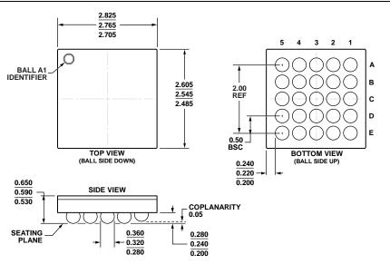
Figure 51. 25-Ball Wafer Level Chip Scale Package [WLCSP] 2.5 mm × 2.8 mm Body (CB-25-1) Dimensions shown in millimeters
