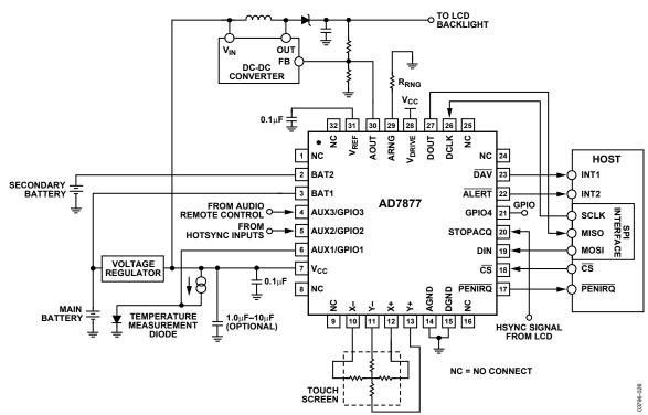
Figure 48. Typical Application Circuit
