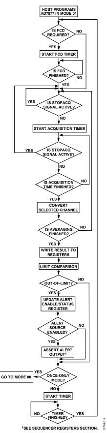
Figure 38. Single Channel Operation
