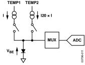
Figure 33. Block Diggram of Temperature Measurement Circuit
