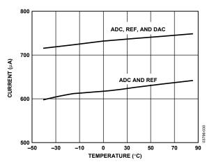
Figure 6. Supply Current vs. Temperature
