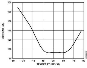
Figure 9. Full Power-Down IDD vs. Temperature
