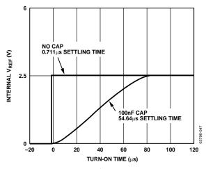
Figure 21. Internal V<sub>REF</sub> vs. Turn-On Time
