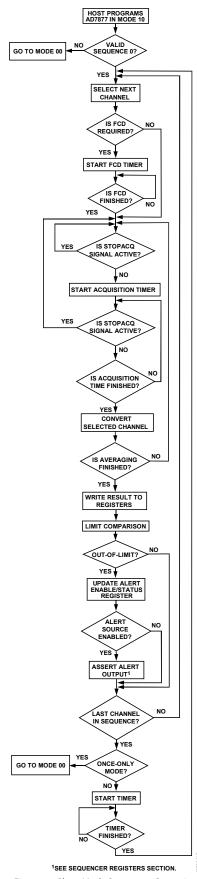
Figure 39. Slave Mode Sequencer Operation
