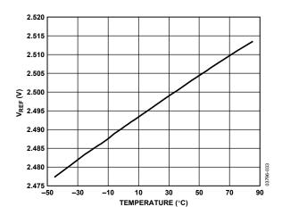
Figure 16. Internal  $V_{REF}$  vs. Temperature
