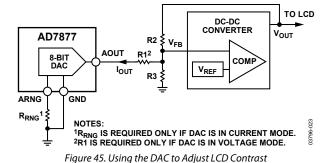
The circuit operates as follows. If the DAC is in current mode when the DAC output is zero, it has no effect on the feedback loop. Regardless of what the DAC does, the feedback loop maintains the voltage across R4,  $V_{FB}$ , equal to  $V_{REF}$ , and the
