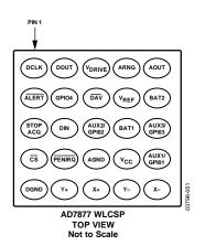
Figure 5. WLCSP Pin Configuration
