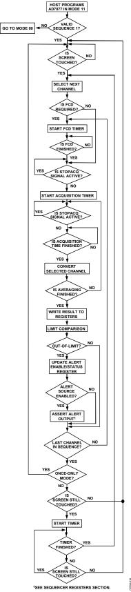
Figure 40. Master Mode Sequencer Operation
