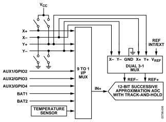
Figure 28. Analog Input Structure
