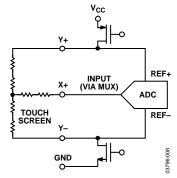
Figure 30. Ratiometric Conversion of Touch Screen Inputs
