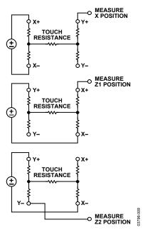
Figure 31. Three Measurements Required for Touch Pressure
