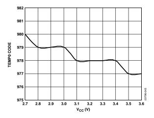
Figure 20. Temp0 vs. V<sub>CC</sub>
