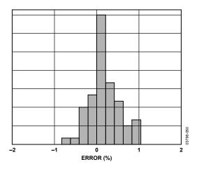
Figure 26. Typical Accuracy for Battery Channel (25°C)
