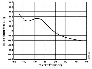
Figure 8. Change in ADC Gain vs. Temperature
