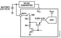
Figure 34. Block Diagram of Battery Measurement Circuit
