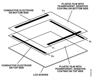
Figure 27. Basic Construction of a Touch Screen
